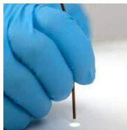
Figure 2: Light pattern from distal tip.
