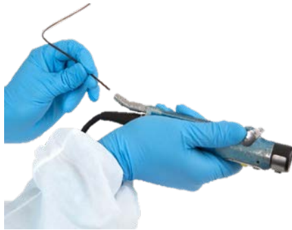
Figure 3: Inserting the scope tip into device.
