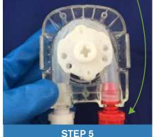
Place the new tube set and rotor inside the pump cap. Properly align the tube set fittings so that they are properly situated in the cap fittings.
