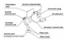
The injector tube (or suction channel tube in this example) is used to inject reprocessing fluids into the instrument channel, suction channel, and air/water channels of the endoscope. It is also used to flush air through these channels to expel fluids.
