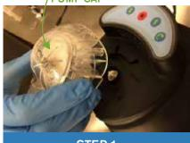
Remove the Pump Cap by pressing on both side tabs and pulling gently.
