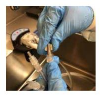
Cap off all unused tubes on the FlexiPump Tube Set. If there are two channels on the endoscope, place a FlexiPump end cap on the end of the third FlexiPump tube lead. If you are flushing only one channel or lumen, cap off the other two FlexiPump tube leads with luer end caps.
