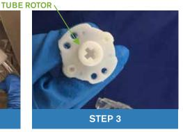
Now that the old set has been taken out, remove the Tube Rotor from the Pump Cap.
