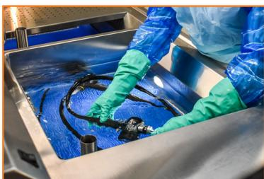
Integrated basin lighting makes leak testing and cleaning easier and more effective
